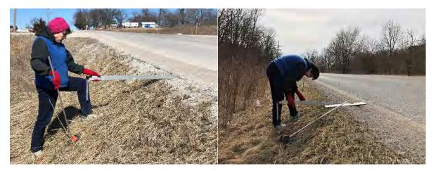
It is worth noting that in several sections of this roadway, there are less than six inches of pavement outside the edge of the white line and there is less than one foot of steep unpaved shoulder. This is typically followed by a drop of over two feet, which is not a "recoverable" slope for vehicles leaving the roadway. At many points along
