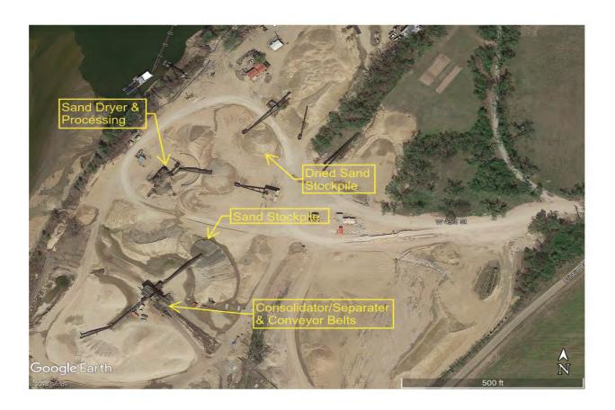
43<sup>rd</sup> & Frisbee Sand Quarry Processing Plant with Consolidator/Separator, Conveyor Belts and Stockpiles
